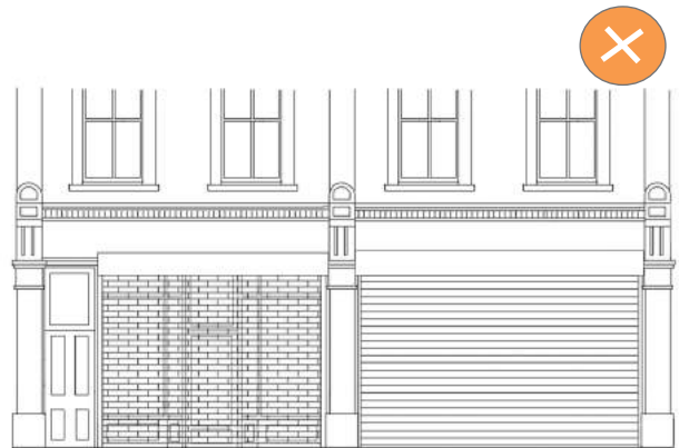
Picture 48. External Roller shutters are not appropriate.
