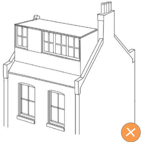
Picture 51. Over-sized dormers will not usually be acceptable in the conservation area.
